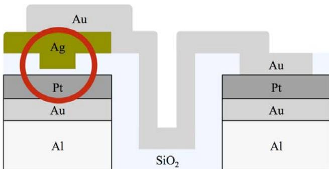
**Figure 5.** Cross-sectional diagram of fabricated structure with active Ag/SiO<sub>2</sub>/Pt area circled. Optical micrograph of top view is in Fig. 6.
