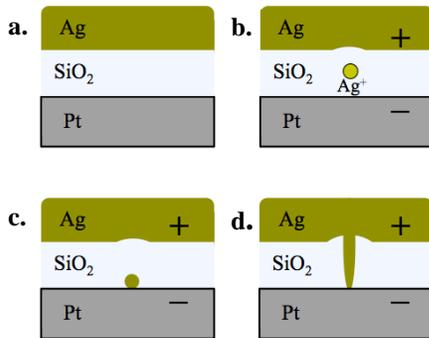
**Figure 4.** Schematic of Ag/SiO<sub>2</sub>/Pt operating principle. The positive bias oxidizes Ag to yield Ag cations (b) that migrate to the Pt electrode where they are reduced (c) until a conductive Ag bridge is formed (d).
