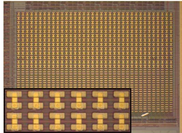
**Figure 6.** Device composition was varied row by row as the fabrication process was optimized. Inset shows devices on the two rows featured in this publication. Pad dimensions are 22  $\mu$ m  $\times$  8  $\mu$ m and 3- $\mu$ m-diameter active device areas are visible on bottom rows.
