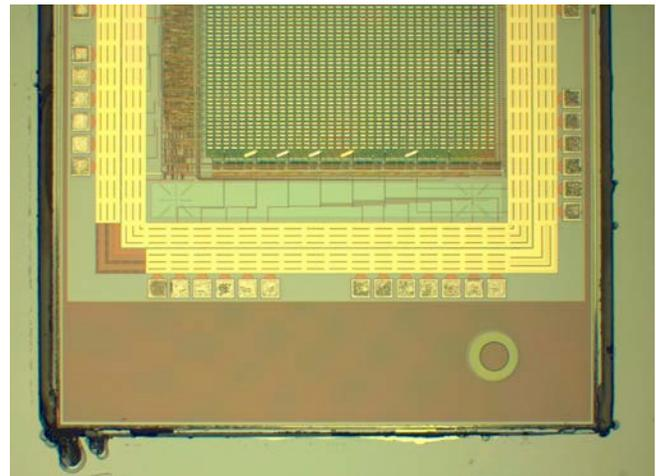
Figure 3. CMOS die integrated in handle after BCB ashing and protection of pads with Au/Pt.
