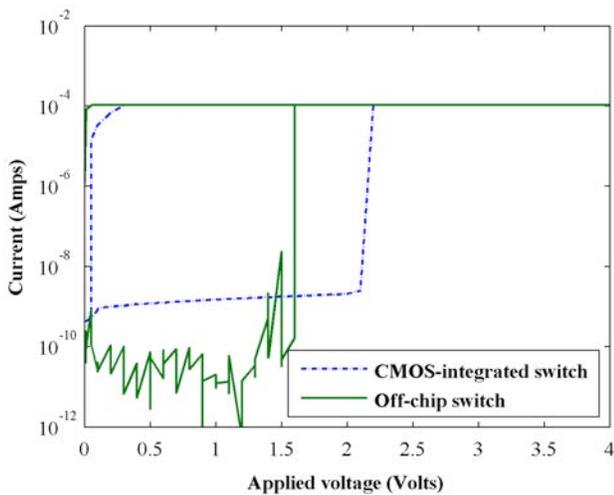
**Figure 9.** Typical positive voltage sweep for CMOS-integrated and off-chip memory. Devices integrated on CMOS have a minimum current level set by the CMOS circuitry.
