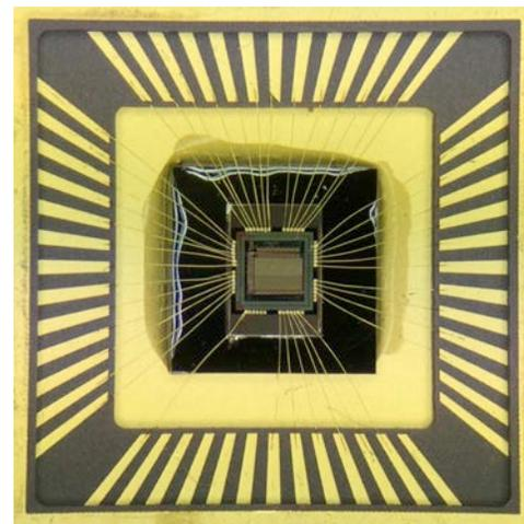
**Figure 7.** Fully packaged hybrid memristor/CMOS die in LCC52.
