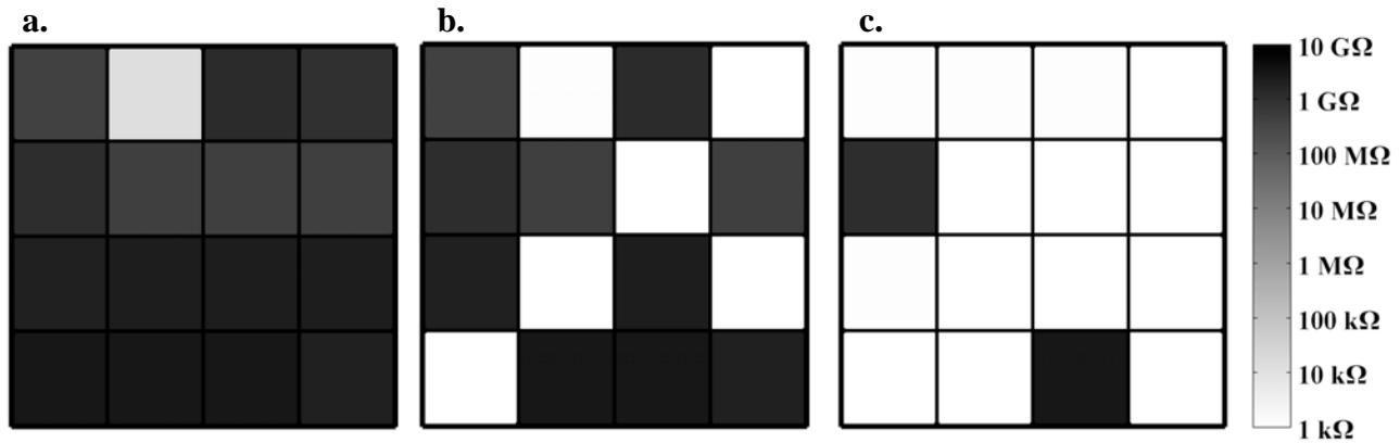
**Figure 8.** Device yield test. Measured resistance of 16 contiguous devices before (a) and after (b, c) 5 V was applied. A checkerboard pattern was programmed (b) followed by its complement (c). Notice one switch was initially shorted (a) and two switches did not change resistance (b and c), corresponding to a yield of 81% (13 of 16).
