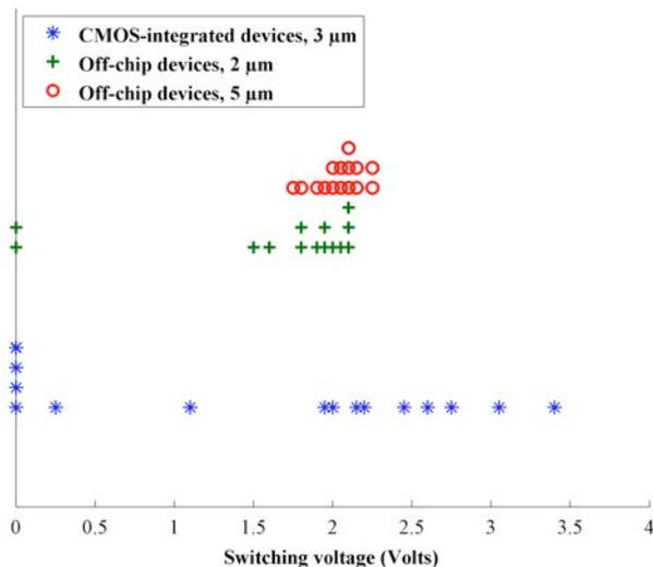
**Figure 10.** Scatterplot of switching voltages. Each dot represents one device. 3- $\mu\text{m}$  off-chip devices were not available for comparison.
