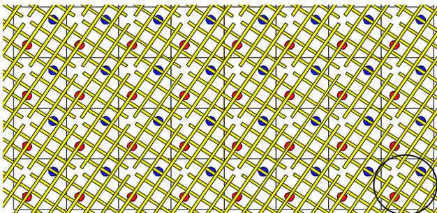
Figure 2. CMOL concept. The circle highlights the CMOS cell, as explained in the text. In this example each red pin is connected to twelve unique memristors. Figure is taken from [24].
