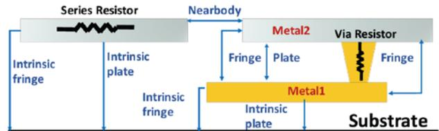
Figure 8. Parasitic resistance and capacitance that can be extracted using layout-parasitic-extraction (LPE) function with PDK.
