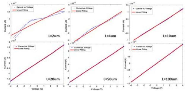
Figure 3. Measured current-voltage ( $I$ - $V$ ) curves (blue-dot) of CNT resistors against linear fitting model (red-line) for resistor length from  $2\mu\text{m}$  to  $100\mu\text{m}$  and the width is fixed to  $40\mu\text{m}$ .
