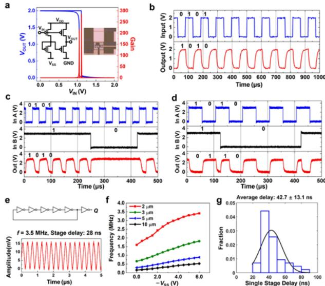
Figure 9. (a) Measured input-output transfer curve and schematics of a *Pseudo-CMOS* inverter. (b-d) measured waveforms of *Pseudo-CMOS* inverter, NAND, and XOR logic gates. (e) measured waveforms of a 5-stage ring oscillator with a large output load 125pF. (f) voltage dependency of the 5-stage ring-oscillator frequencies on the terminal VSS. (g) histogram of the stage-delay using forty-four 5-stage ring-oscillators. The average stage delay is 42.7ns.
