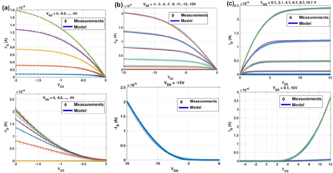
Figure 2. Measured (dotted) and fitted (solid) current-voltage ( $I$ - $V$ ) curves for (a) CNT-TFTs ( $W=125\mu\text{m}$ ,  $L=25\mu\text{m}$ ), (b) Organic TFT ( $W=5000\mu\text{m}$ ,  $L=10\mu\text{m}$ ), and (c) IGZO TFT ( $W=30\mu\text{m}$ ,  $L=20\mu\text{m}$ ) [4].
