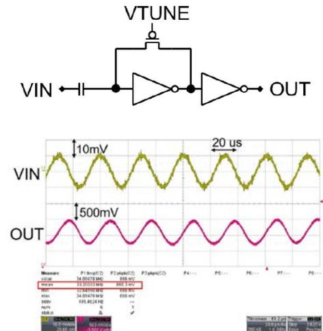
Figure 10. Measured input-output waveforms of a 9T-1C *Pseudo-CMOS* inverter-based VGA with CNT-TFTs.
