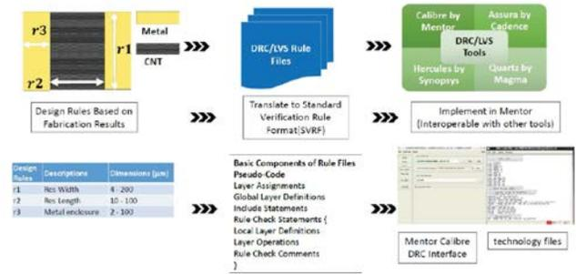
Figure 7. Physical verification flow (ex. DRC) for flexible devices such as a CNT resistor based on experimentally-validated design rules.
