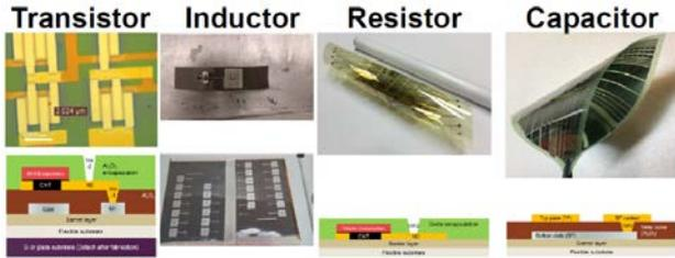
Figure 2. Flexible active and passive devices including CNT TFTs, spiral inductors, CNT resistors, and parallel-plate capacitors.
