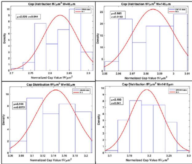
Figure 5. Measured statistical histograms of unit capacitance for the parallel-plate capacitors. The capacitor widths  $W_c$  are from  $45\mu\text{m}$  to  $445\mu\text{m}$ .
