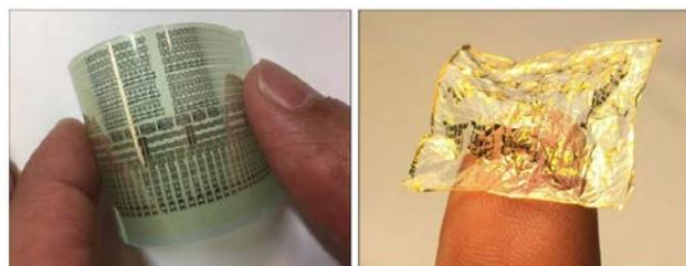
Figure 1. Circuit design IP blocks, including *Pseudo-CMOS* [1] digital logic, analog amplifiers, and passive elements (R/C). (Left) solution-processed CNT-TFT circuits on a 10 $\mu\text{m}$  flexible substrate for bending test, and (right) CNT-TFT circuits on the 1 $\mu\text{m}$  substrate.
