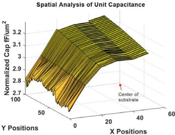
Figure 6. Measured 2D spatial analysis of the unit capacitance ( $\text{fF}/\mu\text{m}^2$ ) against the substrate dimensions in millimeters (mm).
