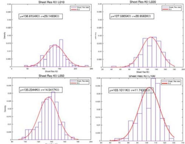
Figure 4. Measured statistical histograms of CNT resistors for resistor lengths from  $10\mu\text{m}$  to  $100\mu\text{m}$  and the width is fixed to  $40\mu\text{m}$ .
