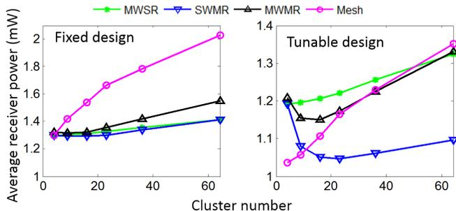
Fig. 13. The average receiver power consumption at different numbers of clusters and for different link structures.
