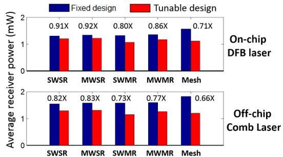
Fig. 14. The average receiver power consumption for different laser types and for different link structures. The numbers denote the ratios of the average receiver power by the tunable design to the fixed design.
