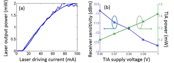
Fig. 6. (a) The laser output power as a function of the driving current of a DFB laser [21] (dots: measurement, line: model); (b) The sensitivity and power consumption versus supply voltage of an adaptive photonic receiver (data from [11]).
