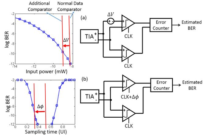
Fig. 8. The two fast BER estimation methods: (a) offset the voltage; (b) offset the sampling time. The data in the left two figures are from [30].
