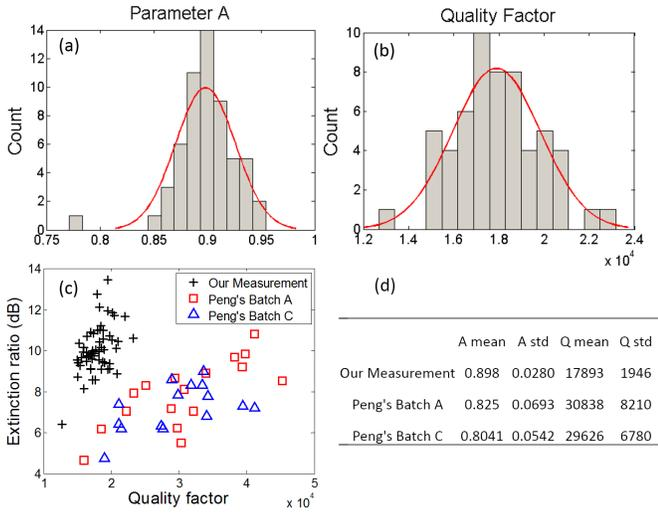
Fig. 3. (a)(b) Histograms of parameters A and Q of our inter-die measurement results; (c) Scatter plot of our inter-die measurement and Peng's intra-die measurement in [18]; (d) Mean and standard deviation (std) of the three measured data sets.
