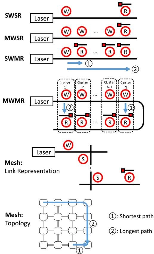
Fig. 9. Five types of link structures. Notions: W: writer or photonic modulator; R: reader or photonic receiver; S: photonic switch or router. In a WDM system, the laser represents a multi-wavelength light source; each microring represents a microring array for multiple wavelength channels
