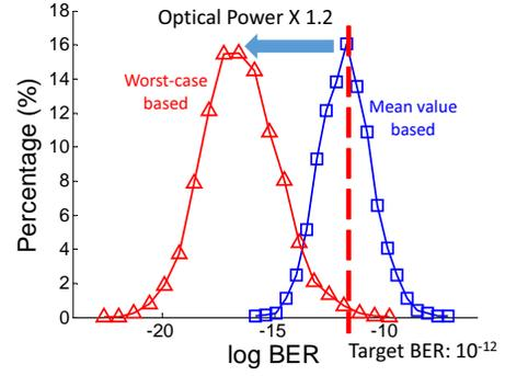
Fig. 5. The BER distribution in the presence of process variations and the electrical tuning. The blue line represents the link configuration based on the means of the device parameters. The red line enhances the link optical power by 1.2X
