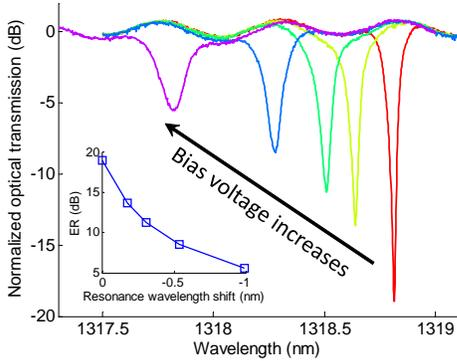
Fig. 4. The measured spectra series of a microring modulator at different bias voltages.
