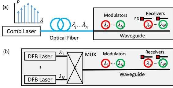
Fig. 1. Schematics of wavelength-division multiplexing (WDM) nanophotonic interconnects using (a) an off-chip comb laser or (b) an on-chip DFB laser array.
