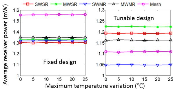
Fig. 12. The average receiver power consumption at different temperature variations and for different link structures.
