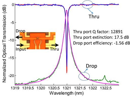
Fig. 2. The optical transmission of the through port and drop port of a microring (blue and green: measurement; red: model). The inset shows a microscopic image of a fabricated microring modulator.
