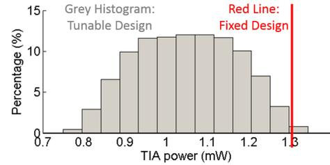
Fig. 10. The simulated TIA power consumption for the fixed design and the tunable design.
