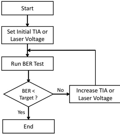
Fig. 7. The adaptive tuning flow.
