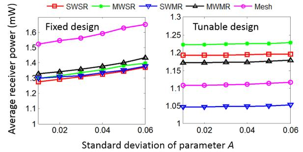
Fig. 11. The average receiver power consumption at different process variations and for different link structures.
