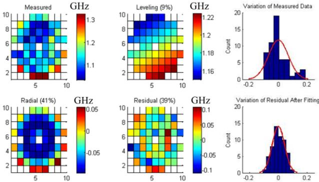
Fig. 3. Measured value and decomposition results of the wafer-scale RC-limited bandwidth.
