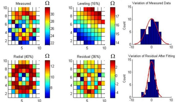
Fig. 2. Measured value and decomposition results of the diode resistance  $R_D$ . The center die is burnt. The radial component is not rotationally symmetric with respect to the wafer center since the DUT deviates from the die center.
