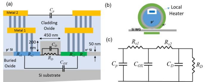
Fig. 1. (a) The cross section of the microring waveguide; (b) The planar view of the microring modulator and the local heater; (c) The small signal circuit model of the microring modulator.
