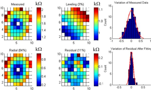
Fig. 4. Measured value and decomposition results of the wafer-scale heater resistance. (Three outlier dies are eliminated.)
