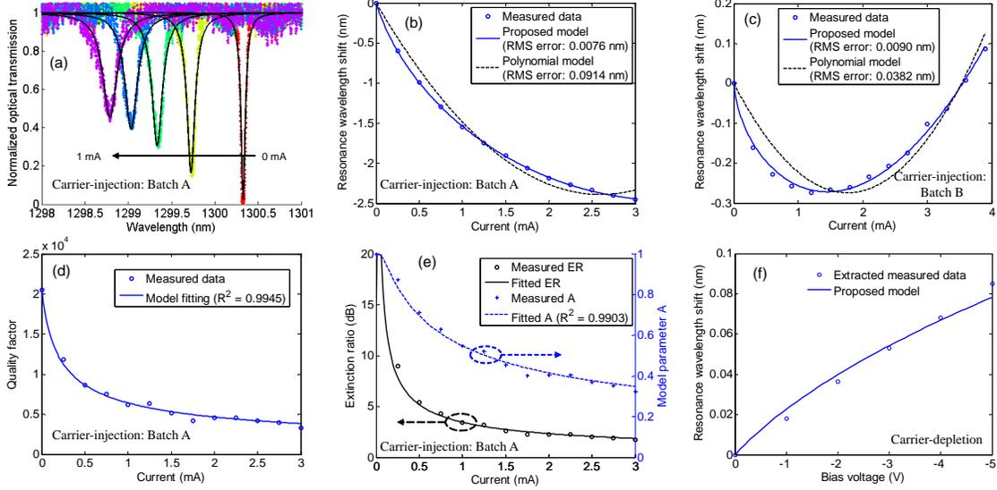
**Figure 5:** (a) Spectra series under injected current ranging from 0 to 1 mA, where dot: measured data, line: modulation model; (b)(c)  $\Delta\lambda_r$  model fitting of carrier-injection modulators from Batch A and Batch B; (d)(e)  $Q$  and  $ER$  model fitting of a carrier-injection modulator; (f) calculated and measured  $\Delta\lambda_r$  (extracted from [22]) in a carrier-depletion modulator.
