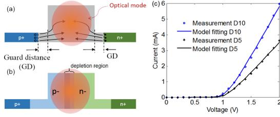
**Figure 4:** (a)(b) cross section views of a carrier-injection modulator and a carrier-depletion modulator, where the guard distance (GD) is the distance between the waveguide and the implantation region. (c) I-V characteristics of two carrier-injection modulators with diameters of 5  $\mu\text{m}$  (D5) and 10  $\mu\text{m}$  (D10).
