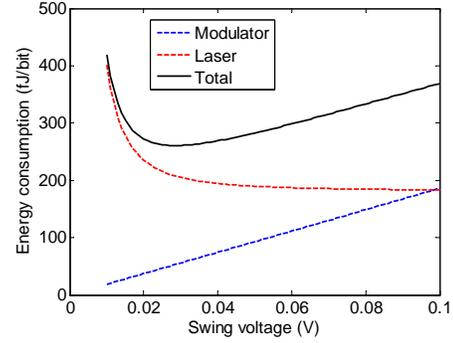
Figure 9: The energy consumption of the laser and the carrier-injection modulator as functions of the modulator AC swing voltage. The DC bias voltage is 1V. The energy consumption per bit of the laser is calculated at a 10 Gbps datarate.
