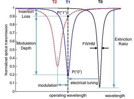
Figure 3: Modulation and tuning scheme of a microring modulator, where the spectrum T0 is at zero bias and the T1 and T2 are respectively transmitting logic "0" and "1".
