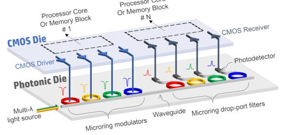
Figure 2: A 3D stack multi-core system using WDM nanophotonic interconnects.
