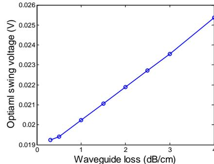
Figure 10: The energy-efficient swing voltage for a carrier-injection modulator as a function of the waveguide loss. Common waveguide loss values (0.3 - 4 dB/cm) are swept [28].
