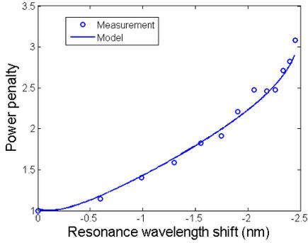
Figure 7: The power penalty for the electrical tuning as a function of tuning distance.
