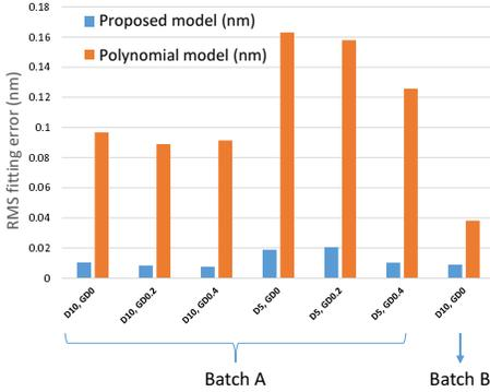
**Figure 6:** Root mean squared (RMS) fitting errors using our proposed model and the polynomial model, where D denotes diameter and GD denotes guard distance illustrated in Fig. 4 (a).
