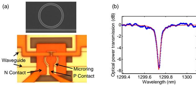
Figure 1: (a) The SEM (upper) and the microscopic (lower) image of a fabricated microring modulator; (b) The measured and model fitted optical transmission spectrum of a microring modulator.
