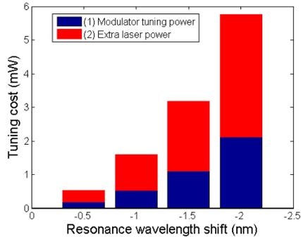
Figure 8: The total tuning cost for the electrical tuning as a function of the tuning distance. The link budget assumptions: receiver sensitivity:  $-17\text{dBm}$  @  $10^{-12}$  BER at 10 Gbps [26]; waveguide loss: 2.5 dB/cm; waveguide length: 1 cm; the silicon hybrid laser wall plug efficiency: 2% [27]
