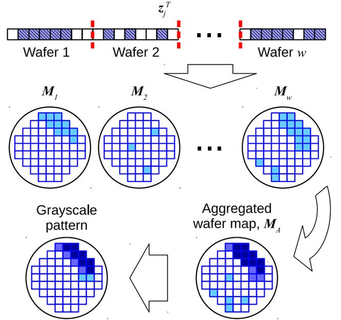
Fig. 6: The procedure of extracting grayscale patterns from a bicluster that is derived by FABIA using WAT data.
