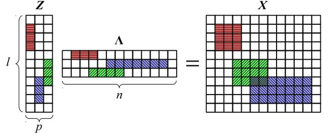
Fig. 2: A multiplicative model with three biclusters. Each rectangular checkerboard represents a matrix. Colored/hatching rectangles are nonzero elements of matrices while white rectangles are zeros. The nonzero elements within a bicluster and within the corresponding prototype and factor vectors have the same color and hatching pattern. Note that the nonzero elements are adjacent to each other for visualization purposes only and additive error  $\Upsilon$  is not shown in this figure.
