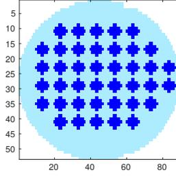
Fig. 8: The mapping between site locations and die locations. Each WAT sample is replaced with 24 die samples in the same region.
