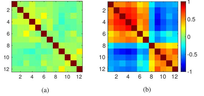
Fig. 10: Linear correlation matrix of twelve WAT items of Bicluster 1. Each rectangle represents a color-coded correlation coefficient of two WAT items. (a) and (b) were derived based on  $S'_1$  and  $S_1$ , respectively.
