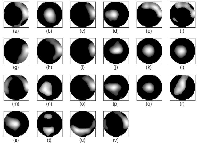
Fig. 11: A grayscale pattern gallery. The intensity of each wafer map is expressed within a range from zero (black) to one (white). Note that the regions outside of a wafer map should be in black (zero values) and are shown as white regions for better visualization.
