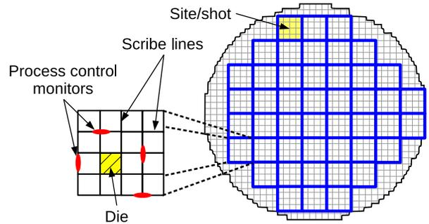
Fig. 4: The spatial relations between sites/shots and dies. Process control monitors are denoted by red ellipses located on the scribe lines. Sites are denoted by rectangles with blue thick edges. Note that the dies close to wafer boundary form incomplete sites that are not emphasized in the figure and are incapable for probing process parameters.
