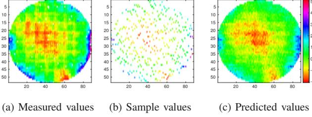
Fig. 1: (a) Measured values, (b) sampled values, and (c) VP-predicted values of a test item from an industrial product. The values are color-coded to produce the wafer maps.
