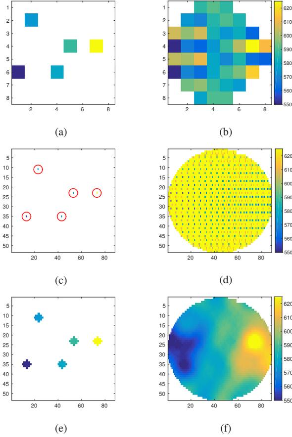
Fig. 5: Color-coded predicted wafer maps of WAT using different sample strategies. (a), (c), and (e) show the samples, as a single site, a single die, and multiple dies, respectively, used by VP for prediction/extrapolation. (b), (d), and (f) show the corresponding predicted wafer maps.
